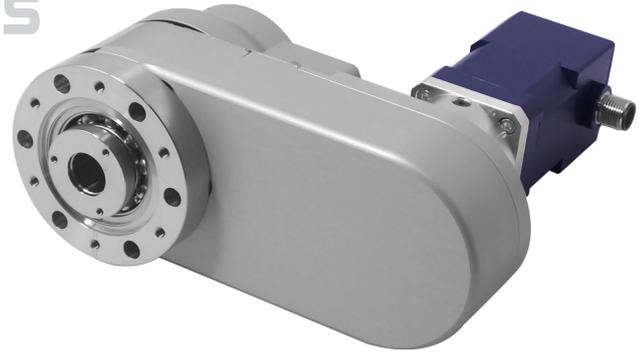
MD40H is a high torque, medium stiffness rotary drive. Configured with a hollow body, the MD40H has a fixed rear flange enabling a component to pass through the centre, such as a heater module, a feedthrough, a second MagiDrive rotary feedthrough or a cold lance.
