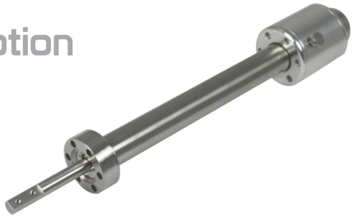
Unguided linear motion solutions for low load applications in high/ultra-high vacuum. The vacuum shaft is free to rotate, avoiding possible conflict with an internal chamber mechanism. Available in CF16 and CF35 flanges and six stroke lengths from 50mm to 300mm. Manual, pneumatic and motorised actuation options with additional switches to prevent over-travel.
