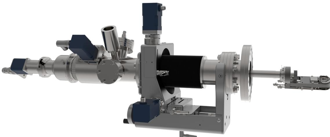
XL-T | 5-axis manipulator utilising hollow and solid magnetically-coupled rotary drives to provide Polar (R1) and Azimuthal (R2) rotation
